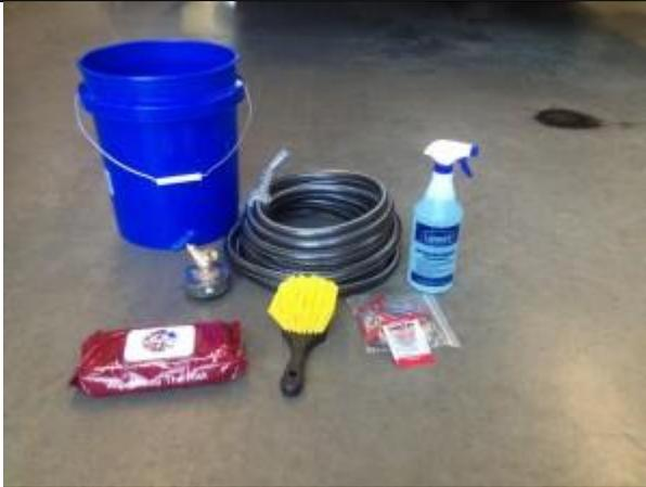
*The Roanoke Fire-EMS Department's decon equipment includes: 5 gallon bucket, 25 feet of garden hose along with 2 ½" blind cap and garden spigot added to it, scrub brush, bottle of turnout gear washing spray, wet wipes, and individual packets of SPF 30 to be used while out training or during long-duration incidents.*
